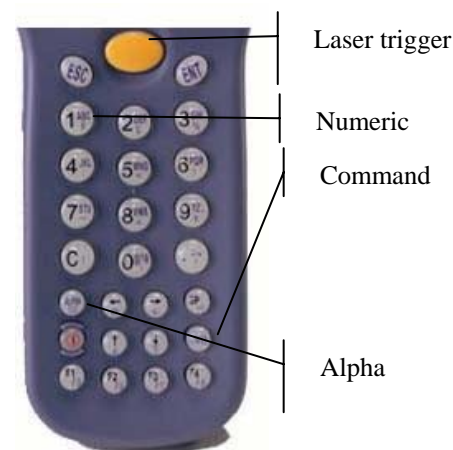
Figure 0-9: HT630 Keypad Legend
